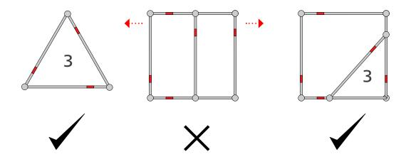
Structures should be firm and stable. Squares are not stable. Triangles are.
